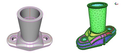
Figure 1: Meshing of a NURBS model where one can see the singularity graph which is protected within a collection of spheres.
