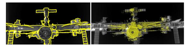
Left. Example of ISS tracking in images, where the 3D model is accurately known a priori. Right. Example of LiDAR data acquired on the ISS. Both camera and LiDAR data have been acquired during the LIRIS experiment on ATV-5.
