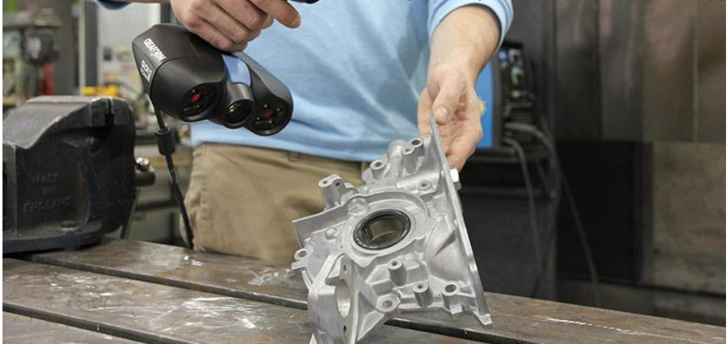
Fig 1. A Go!Scan3D (<https://www.goscan3d.com/en>) portable point cloud scanner
